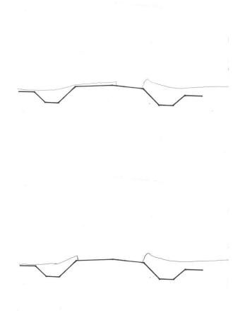
As we begin to plow the snow, we compound the problem on the windy side of the road, because we try to throw the snow into the wind. We end up going slow because visibility is low. Consequently, the bank keeps getting higher and harder.
