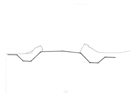
By the time we get to the bank with the grader wing, the damage is done, and we have high, straight walled banks. If left like this, they will fill in every time the wind blows. If we just continue to plow them, soon they will be unmanageable with a plow truck. Remember, we have probably added de-icing chemicals to the road, then plowed them onto the bank. This makes the banks much harder.
