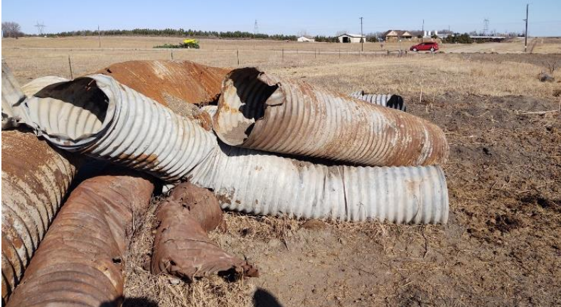
Site: ZeHor09, Culverts that were replaced awaiting to be relocated to recycling center off 27th AVE NE, 2019-05-09 Pic 3 of 3
