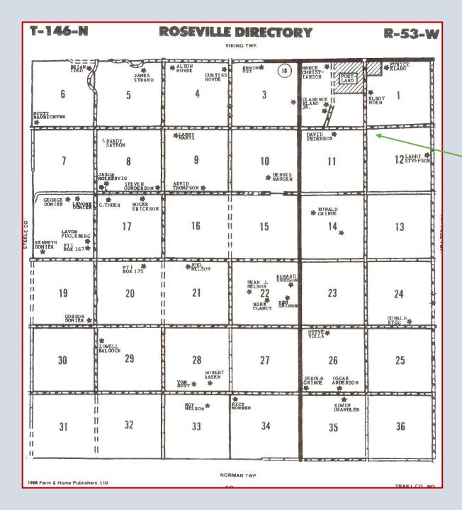
The grid seen on this map shows the section lines, (the boundaries between the one- mile square sections of land).
