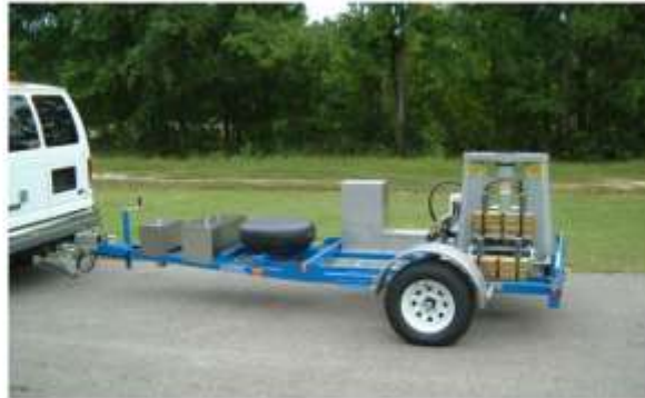
Figure 2. Dynatest 8002 FWD Test System.
