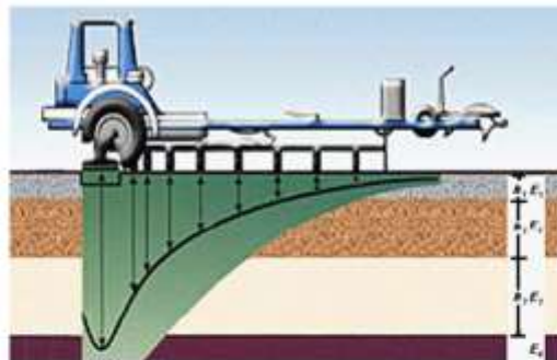
Figure 3. Schematic representation of FWD testing.
