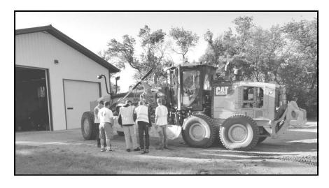
operator instructor suggested adding a 2-foot extension to the moldboard to bring it to 16 feet in length, making operators more efficient in blading the roads.
