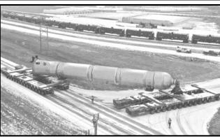
thon Oil hired an engineering firm and worked with the county and NDDOT Bridge Division to analyze the bridge to assess if it on the capacity to withstand the load. In the end, three bridge analyses were done before the movements were approved by the county and permits could be issued.
